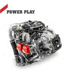
SKYRUNNER is equipped with duel power systems, one for ground transport and one for air. The Rotax 914 UL – the same engine used in the U.S. Air Force's MQ-1 Predator – features 160 hp that when paired with ram-air parafoil wing technology gives the SkyRunner a flight range of 140 nautical miles and a maximum air speed of 45 mph.
